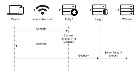
If the user has selected "Maintain general location," the user's device will share the geohash information with the second internet relay. This information allows the second internet relay to select a representative Relay IP address from a pool of addresses assigned to the location.
