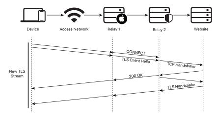
In networks where QUIC traffic is blocked, devices use the CONNECT method of HTTP/2 to communicate with the proxies, with the same requirement for TLS 1.3 and raw public keys.
